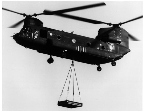
*Figure 1 CH-47D with a Single-Point External Load.*
